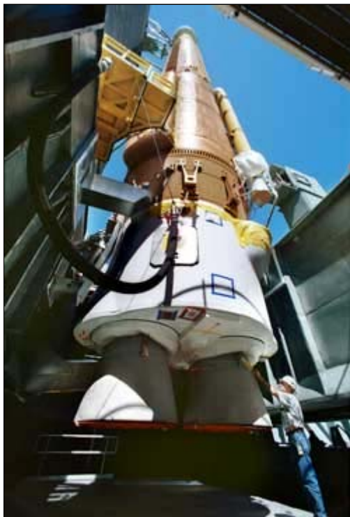
A view looking up at the Atlas 5 from beneath the mobile launching platform at Cape Canaveral. The bar-like structure extending from the left of the platform to the rocket is one of the three hold-down posts. The box-like mast on the platform's deck to the right of the rocket is where the first stage liquid oxygen is loaded into the vehicle along with other umbilicals. Photo: Lockheed Martin
