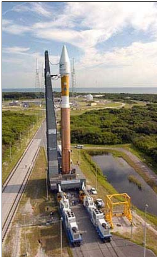
Atlas 5 rocket on its mobile launch platform. Photo: Lockheed Martin
